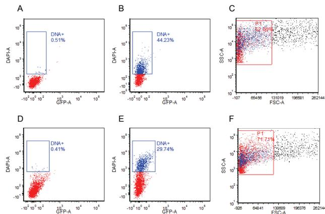
Fig. 7. Flow cytometry results from test samples. Top panels (A-C) and bottom panels (D-F) represent two individual test samples. (A and D) Background DAPI emission versus green fluorescent protein (GFP) emission for samples without DAPI added. (B and E) DAPI emission versus GFP emission for samples following the addition of DAPI. (C and F) Side scattering (SSC) versus forward scattering (FSC) for samples following the addition of DAPI; FSC represents an index of particle size.
