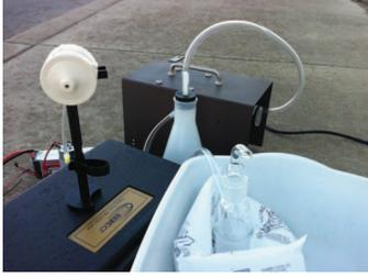
Fig. 2. Liquid Impinger and SS2 test
