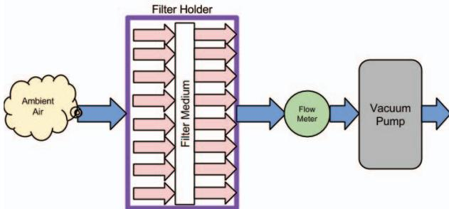
Fig. 1. SS2 Air Sampling unit
