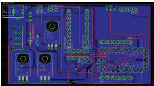
Fig. 8. PCB Schematic for SS1 v2
