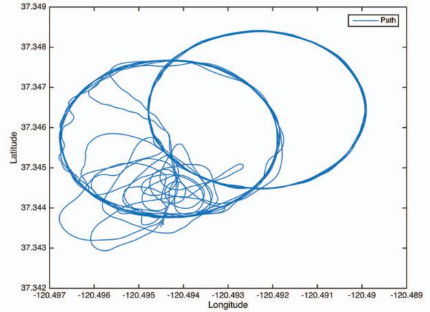
Fig. 4. Flight path of SDD1. Two intersecting circles indicate the flight paths of a sampling operation. The left circle is the first portion of the sampling cycle, and the right circle is the final portion.
